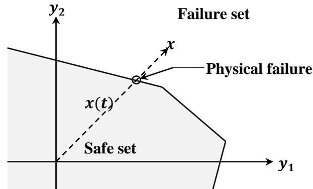
Figure 4.17 Multiple linear limit states after shaping and straight load evolution function
