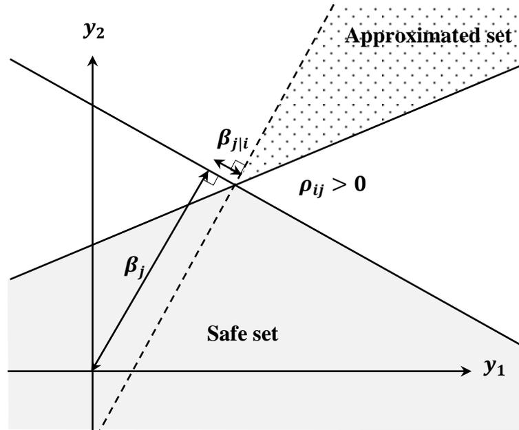
Figure 4.22 Failure set corresponding to the probability  $\phi(-\beta_j) \cdot \phi(-\beta_{i|j})$
