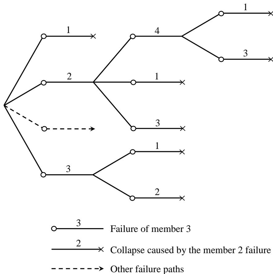
Figure 2.7 Failure paths tree
