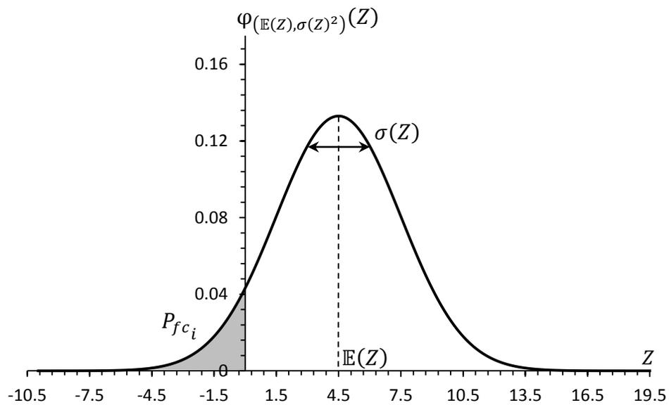
(b) Normal distribution of  $Z$ Figure 3.8 Member probability of failure associated with  $Z$
