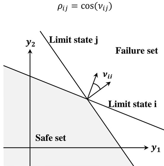
Figure 4.23 Geometric interpretation of the correlation coefficient  $\rho_{ij}$  [2]
