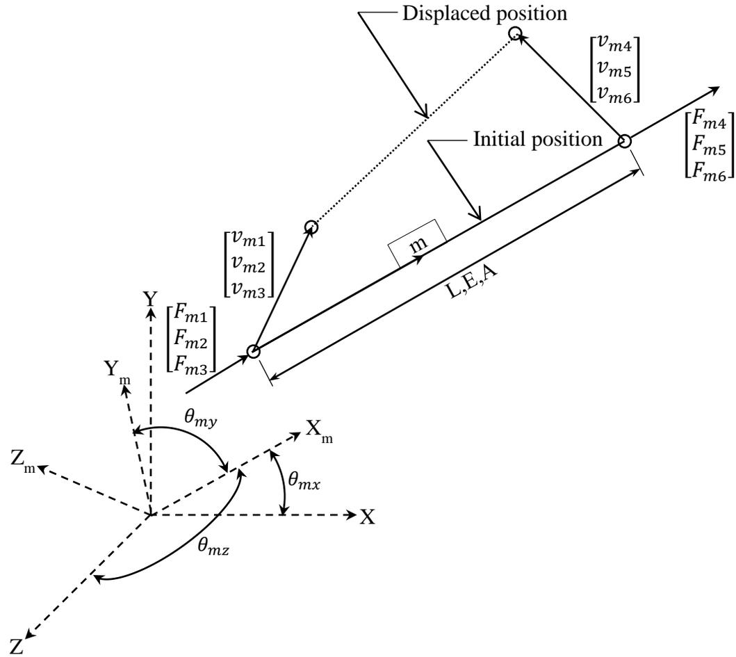
Figure 3.4 Member forces and displacement in the global system and relationship between the local and global coordinate system
