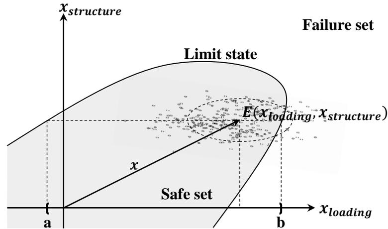
Figure 4.29 Linear limit state approximation and variables scatter
