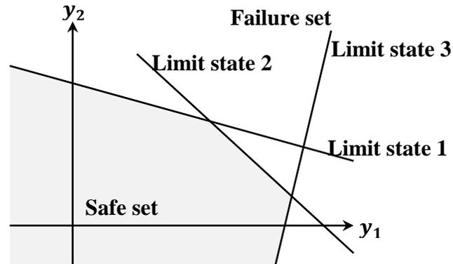
Figure 4.16 Multiple linear limit states before shaping
