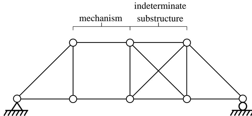
Figure 2.1 Truss structure with a mechanism and an indeterminate substructure
