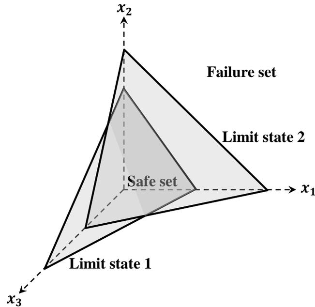
Figure 4.6 Multiple linear limit states in 3-dimensional space
