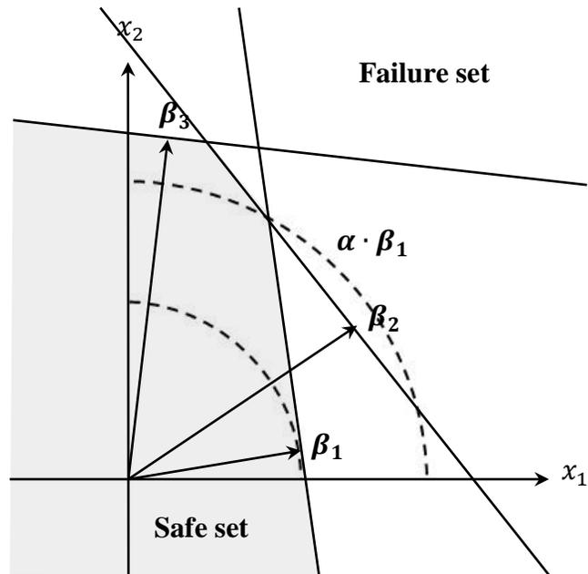
Figure 4.12 Reliability model with unnecessary limit states
