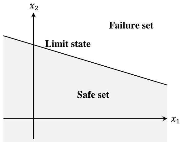
Figure 4.2 Linear limit state
