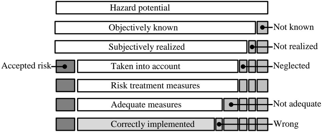
(a) Origins of the risks for a structure with low levels redundancy
