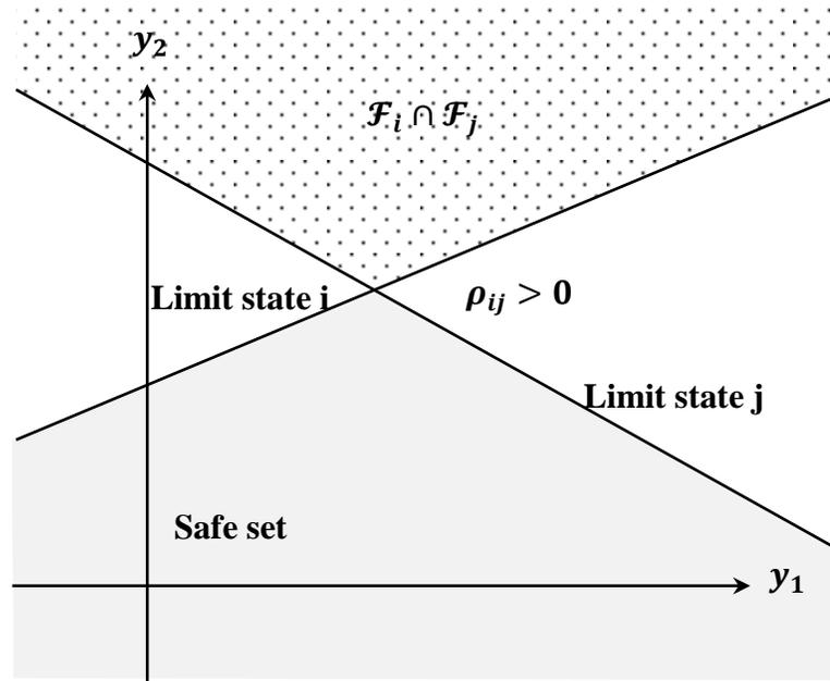
Figure 4.20 Joint failure set for the limit state i and the limit state j
