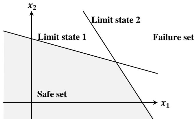
Figure 4.5 Multiple linear limit state in 2-dimensional space
