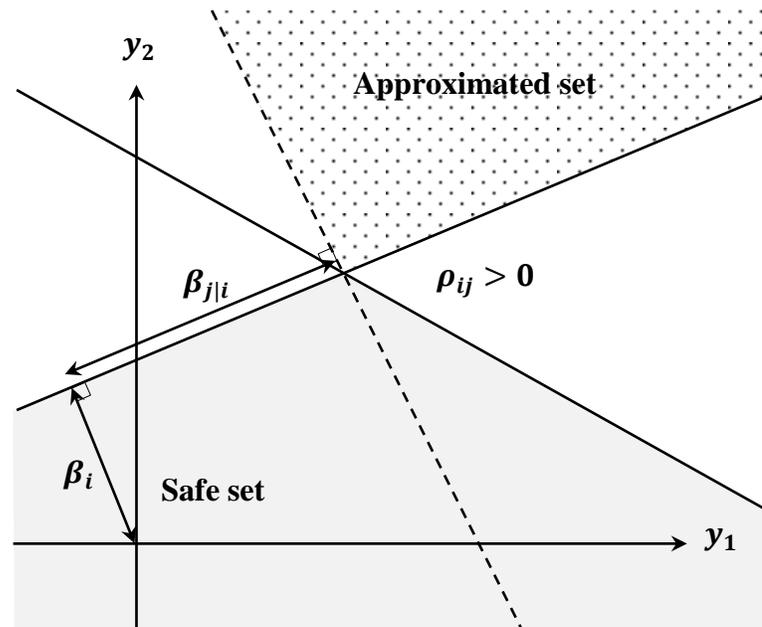
Figure 4.21 Failure set corresponding to the probability  $\phi(-\beta_i) \cdot \phi(-\beta_{j|i})$
