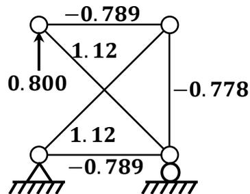
Figure 5.7 Forces in members caused by the member 1 plastic force
