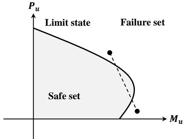
Figure 4.4 Non-convex failure set for a concrete column.
