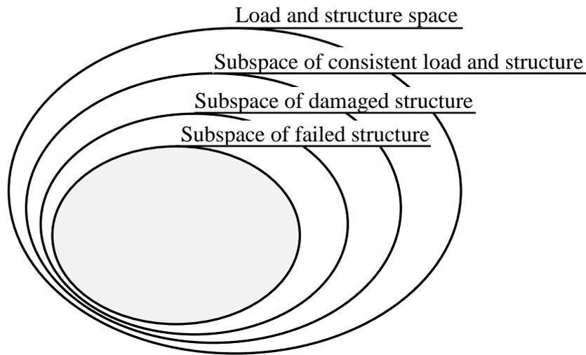
Figure 2.10 Venn diagram of the load and structure space
