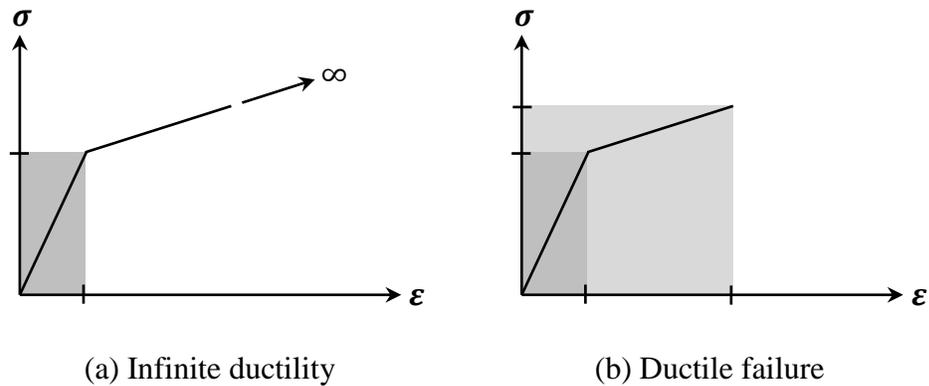
Figure 4.25 Linear elastic – linear work hardening model
