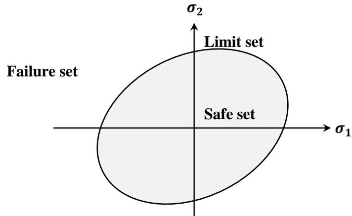
Figure 4.1 Von-Mises Criterion limit state
