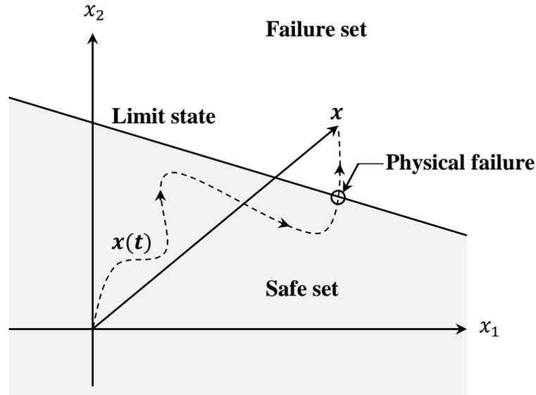
Figure 4.9 Loading evolution function in the subset  $\mathcal{Q}$
