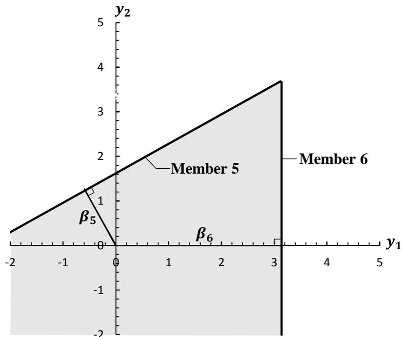
Figure 5.9 Consistent limit states for the structure with member 1 failed
