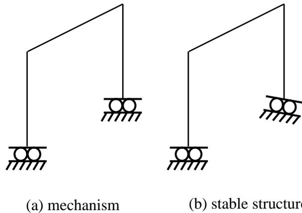
Figure 2.2 Comparison of two structures with one degree of redundancy
