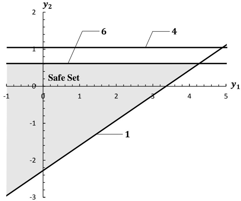
Figure 5.12 Limit states in the normalized space for the structure with member 3 failed
