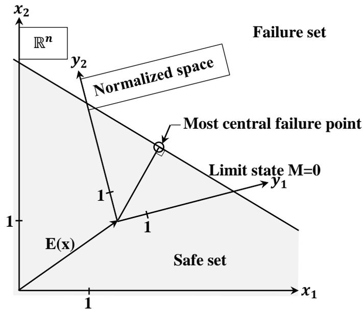
Figure 4.14 Most central failure point
