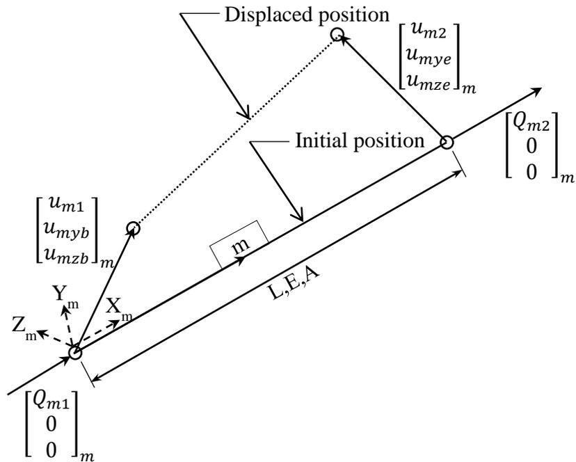
Figure 3.3 Member forces and displacement in the local coordinate system
