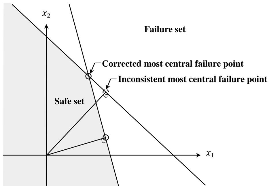
Figure 4.15 Most central failure points for multiple limit states
