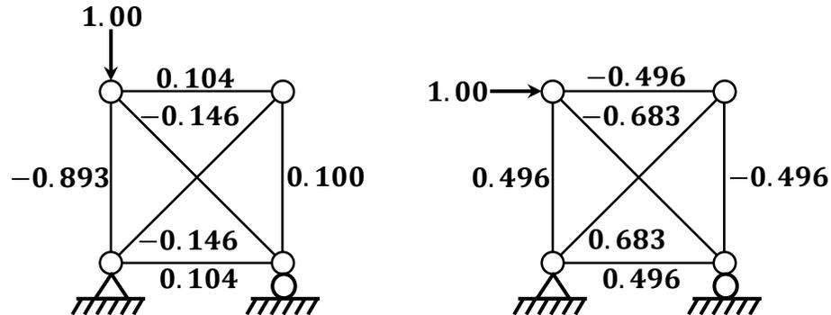
Figure 5.2 Results of the structural analysis for the intact structure
