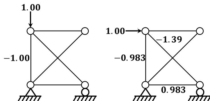
Figure 5.10 Results of the structural analysis for the structure with member 3 failed
