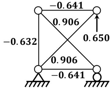
Figure 5.11 Forces in members caused by the member 3 plastic force
