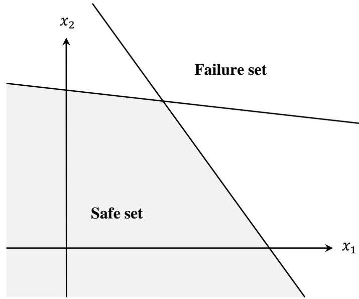
Figure 4.11 Corrected reliability model without inconsistent limit states
