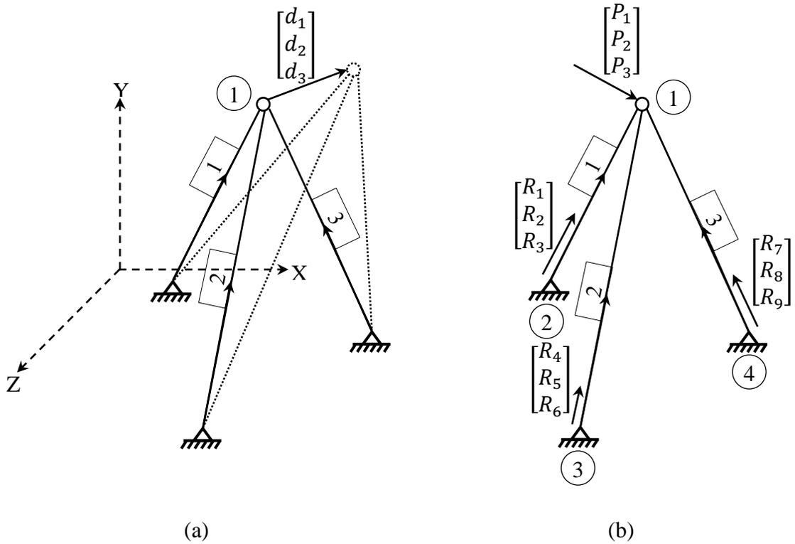
Figure 3.5 Displacement vector, load vector and reaction vectors
