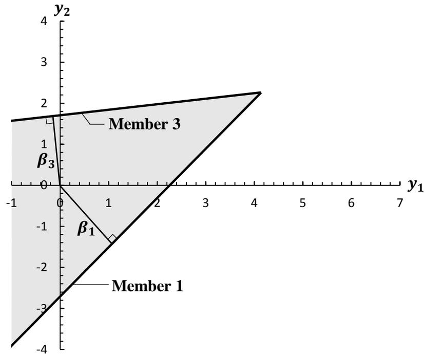
Figure 5.5 Consistent limit states for the intact structure
