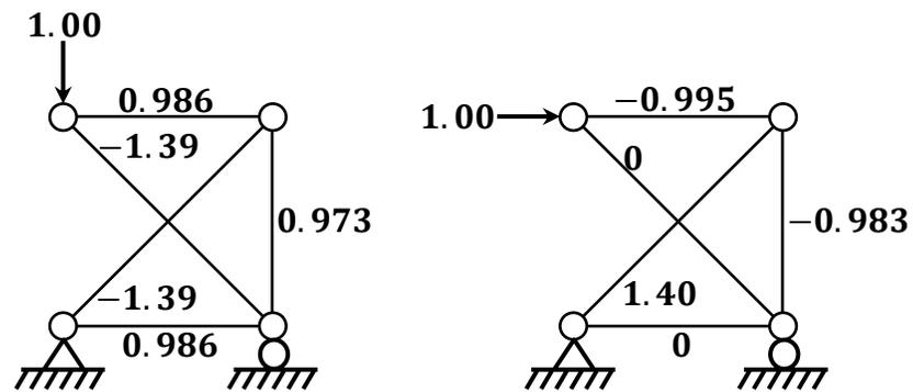
Figure 5.6 Results of the structural analysis for the structure with member 1 failed
