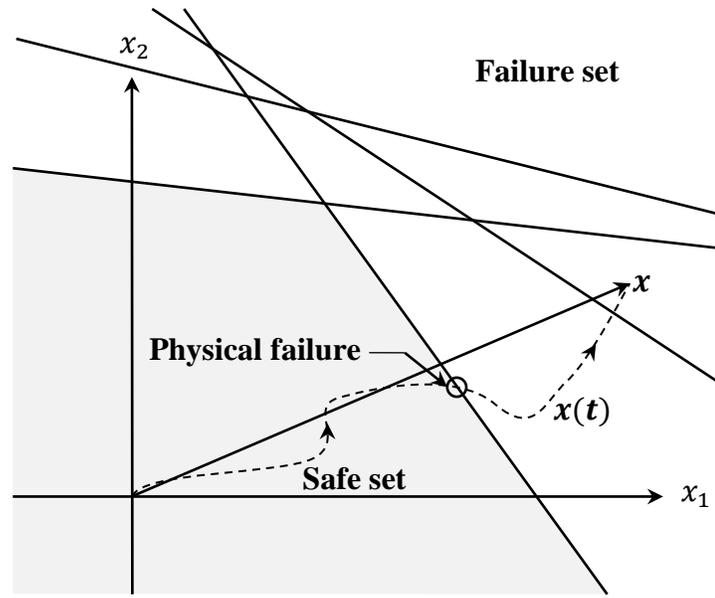
Figure 4.10 Reliability model with inconsistent limit states
