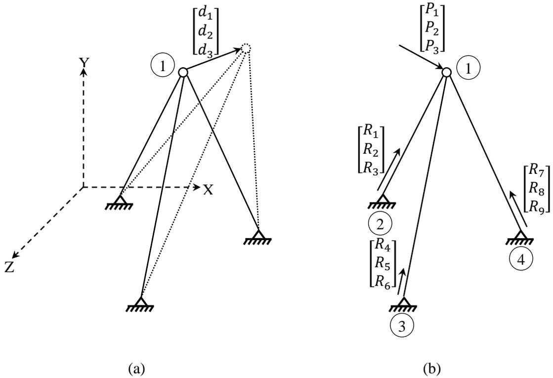
Figure 3.2 Degrees of freedom, joint load vector and reaction vector
