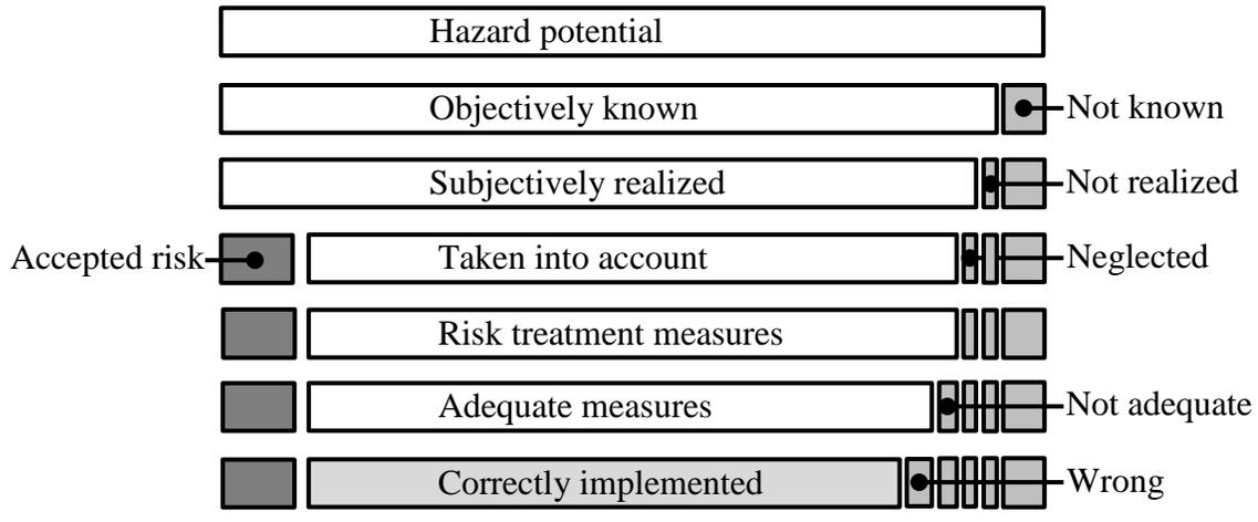
(b) Origins of the risks for a structure with high levels
