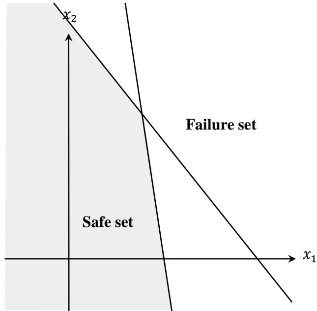
Figure 4.13 Corrected reliability model upon removing unnecessary limit states
