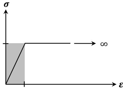
Figure 4.24 Linear elastic – perfectly plastic model
