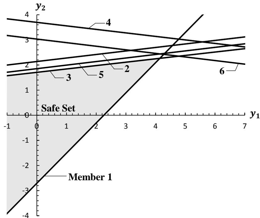
Figure 5.4 Limit states in the normalized space for the intact structure
