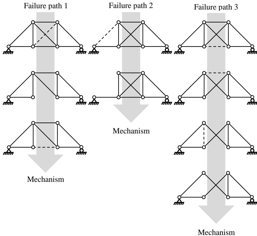
Figure 2.6 Failure paths
