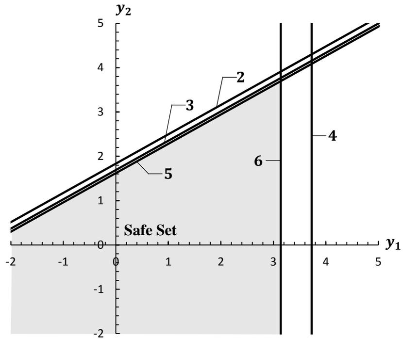
Figure 5.8 Limit states in the normalized space for the structure with member 1 failed
