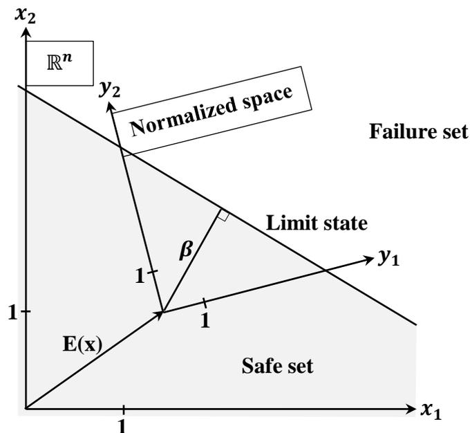
Figure 4.7 Geometric interpretation of the reliability index in the normalized space
