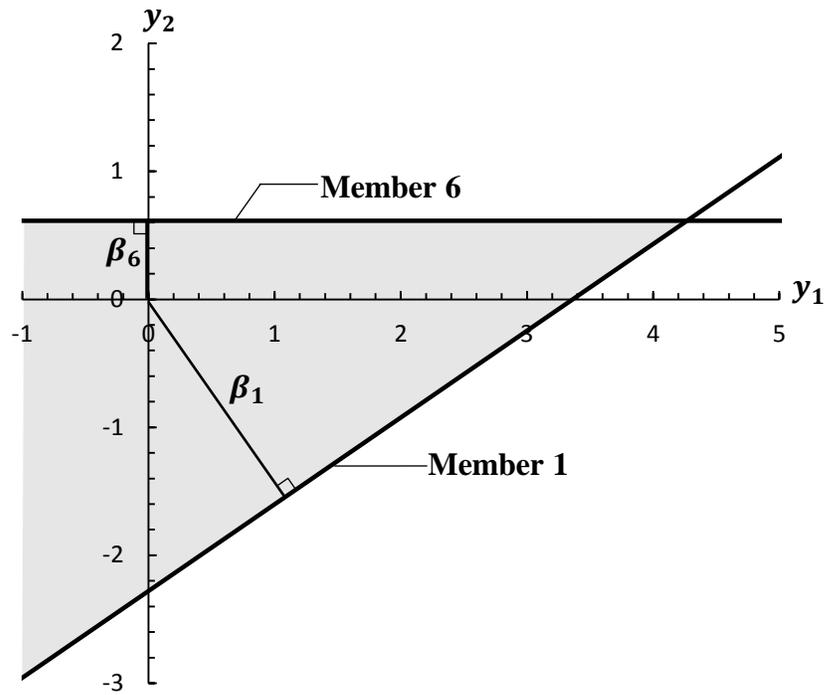
Figure 5.13 Consistent limit states for the structure with member 3 failed
